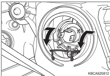
**10** 電球を取り外す
